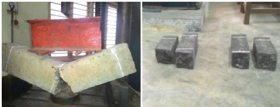
Fig.3.5 Beam specimens after testing for flexural strength
