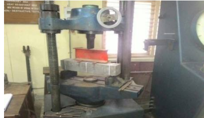
Fig.3.4 Beam specimen on universal testing machine (UTM)
